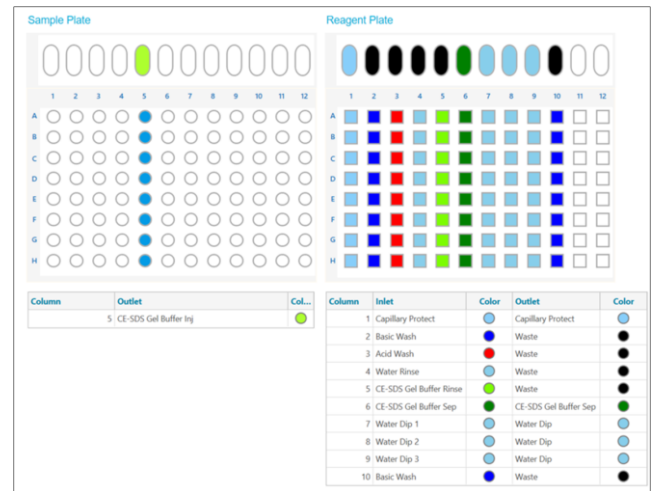
Figure 5. Sample and reagent plates layout generated by the BioPhase software. This representative layout indicates that 8 samples (column 5, left side) were analyzed using the loaded CE-SDS proteins analysis kit reagents as shown on the reagent plates section (right side).
