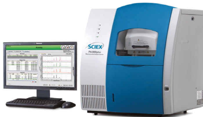
Figure 1: The PA 800 Plus Pharmaceutical Analysis System with laser induced fluorescence detection (CE-LIF).
