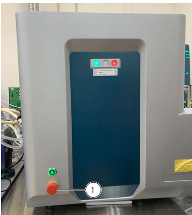
Figure 6-1 Emergency Off Switch on the Front Panel of the Echo ® MS Module
