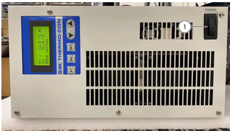
Figure 4-3 Chiller Module Convenience Switch
