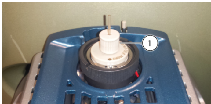
Figure 3-3 Lower Fitting Installed
