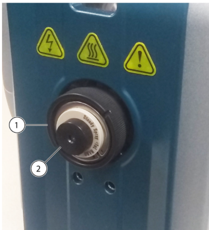
Figure 3-13 Union Installed in the Nano Probe
